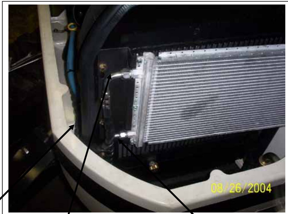
5/16" 90° fitting on the bottom outlet of the condenser.
