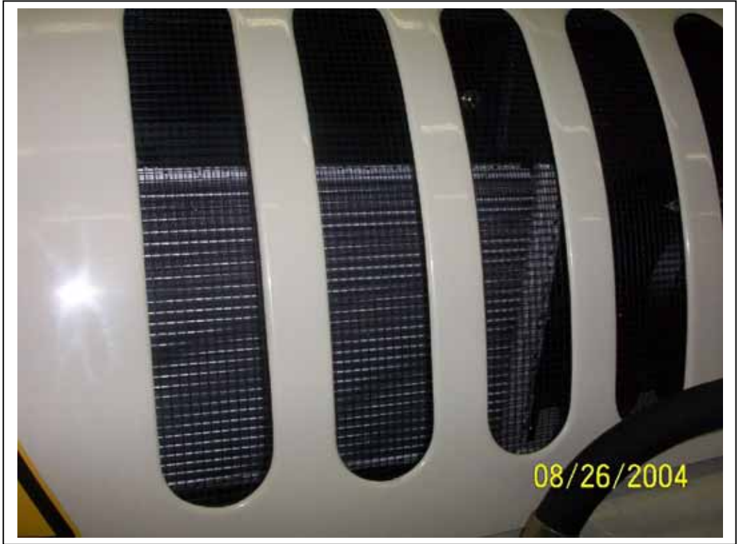
Condenser in place with the hood down
