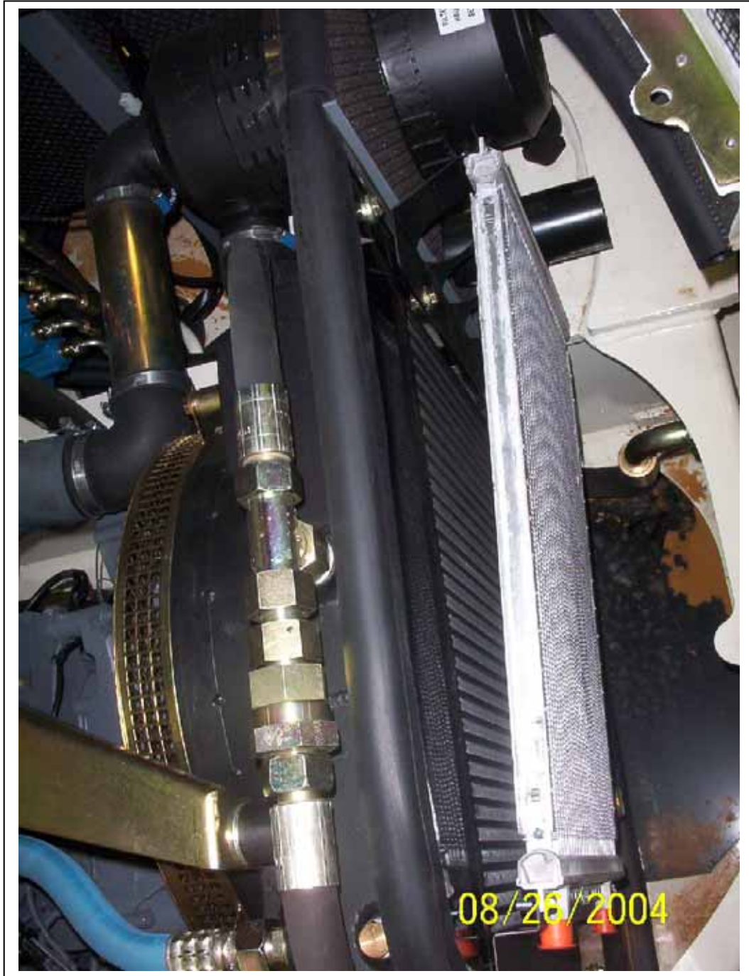
The condenser frame is angled to allow for easy cleaning and maximum air flow across the radiator.
